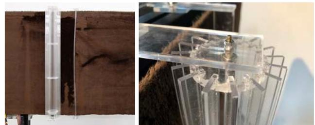
Figure 4: Reset system with roller and guide(left), and reset roller(right)
