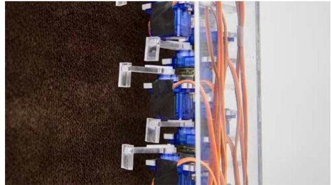
Figure 3: Arrangement of 30 servomotors designed to generate 30 compact lines.
