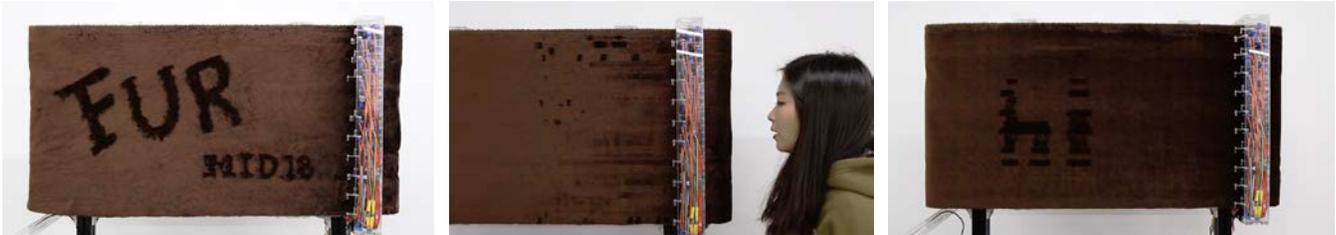
Figure 1: Three ways to input graphics on FurPlay: a) hand drawing, b) user's voice, and c) preset on servomotors.
